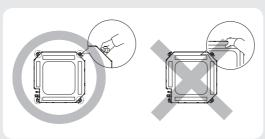
Do not hold the discharge while carrying the indoor unit to avoid the possibility of breakage. You must hold the hanger plate on the corner and carry the indoor unit.
