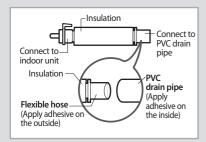
◆ Handle with using adhesive not to block the inside of flexible hose
