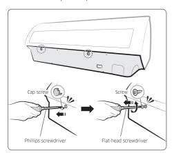
2 Unlock the side hooks (1), 2), then centre hooks (3). Then unlock the bottom hooks (3) to pull out the cover panel.
