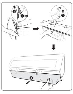
Step 2.2 Disassembling the installation plate
