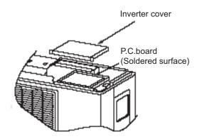
(2)As shown below,connect the discharge resistance(approx.100 $\Omega$ 20W)or plug of the sold ering iron to voltage between + - terminals of the electrolytic capacitor (test3 "D" and "E" point) on PC Board for 30s, and then peformedischarging.
