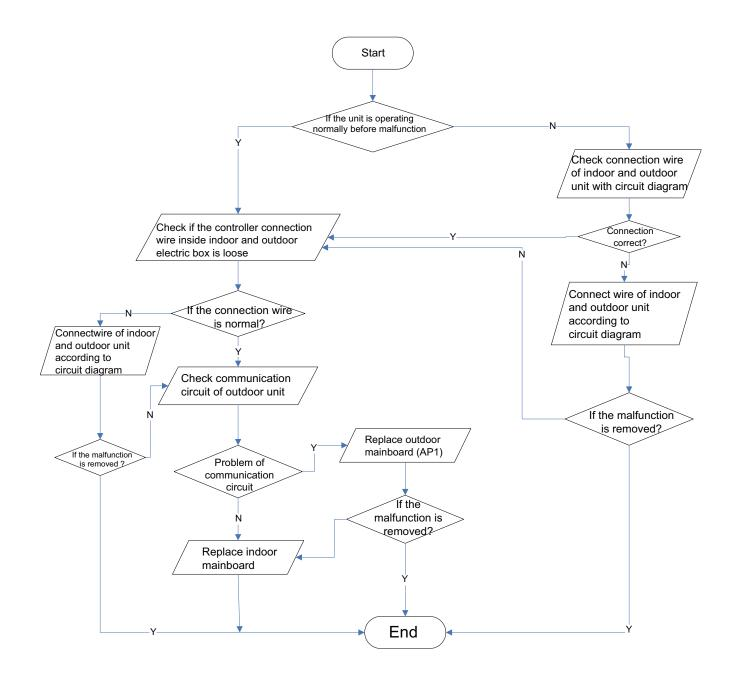
Diagnosis process for outdoor communication circuit (refer to the key detection points of outdoor unit)
