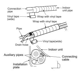
4. Bundle the piping and drain hose together by wrapping them with vinyl tape for enough to cover where they fit into the rear piping housing section.
